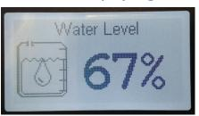
This page displays the current water level in the leisure vehicle as a percentage. If the "Low Water" notification is enabled the user will receive a notification when their water tank levels drop below 10% by default.
