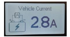
This page displays the amount of current being drawn from the Vehicle Battery, when the Vehicle Battery is being charged a lightning icon is displayed inside the battery. A higher current will draw will drain your battery faster.
