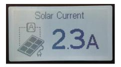
This page displays the amount of current that is being generated by the solar panel. A solar regulator is required to drop down the solar panel voltage to battery safe levels.
