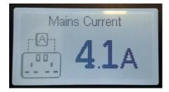
This page displays the amount of current that is being drawn from the 230V mains connection.
