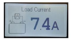
This page displays the amount of current that is being used by the leisure vehicle to power its internal systems, such as lights, pumps and sockets for example.
