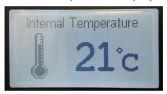
This page displays the internal temperature, it is measured by a sensor inside the control panel and displayed on the screen in degrees Celsius by default.
