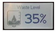
This page displays the current waste water level inside the waste tank as a percentage. If the "High Waste" notification is enabled the user will receive a notification when their waste tank fills up over 90% by default.
