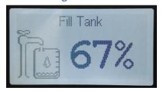
This page is the fill tank screen. When the external pump is connected to the inlet and to an external water source pressing the  $\[ egin{align*} \end{align*} \]$  button will begin filling the internal tank. When the internal tank is full the pump will stop automatically.
