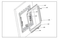
Fit bracket lining up bracket holes with window holes, apply screws to bracket. **Do not over tighten!**
