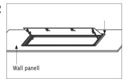
Apply silicone or foam type around window edge and then fit window onto wall. Recommendation:
