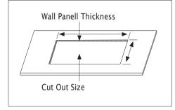
The wall thickness for window must be between 25–40 mm.
