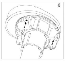
Tighten the ring nut on to the wedge spacer by using two 2.9X13 mm selftapping screws (screws not supplied)
