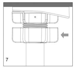
This **mast locking** device must be screwed tight every time you wish to secure the antenna in the desired position. To turn or lift the mast, loosen this ring nut.
