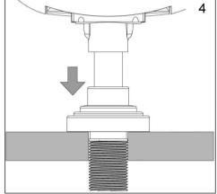
Place the rubber gasket over the ring nut.
