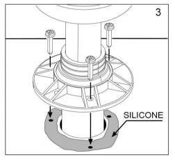
Insert the mast in the hole  $\emptyset$  42 mm bored in the roof, making sure you apply a layer of silicone under the ring nut. Fasten the ring nut using self-tapping screws (screws not supplied).
