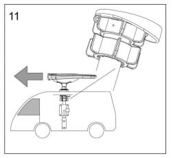
When the vehicle is running, always remember to set the antenna in the position shown in the drawing and to tighten the mast locking device.
