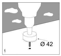
Bore a hole  $\emptyset$  42 mm in the desired position on the roof of your caravan or motor home.
