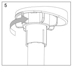
Secure the pipe lead to the roof using the ring nut and its wedge-shaped spacer. Caution: the antenna must be in horizontal position. The wedge-shaped spacer is used to set the antenna in the horizontal position even if the roof is inclined.
