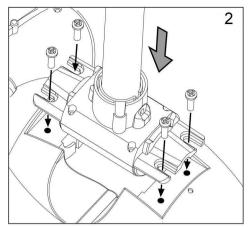
Fasten the mast to the antenna using the four provided screws.
