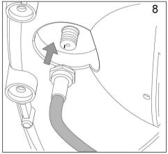
Screw the coaxial cable into the antenna connector.
