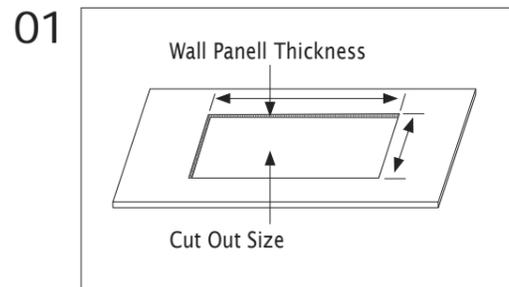
The wall thickness for window must be between 25–40mm.
