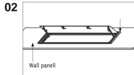
Apply silicone or foam type around window edge and then fit window onto wall. Recommendation:
